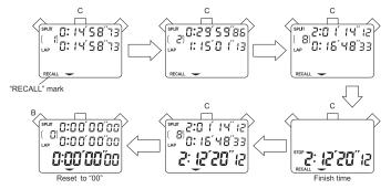
\* To stop the recall of the stored data, press "B" or "D". The measurements when the stopwatch was stopped will be shown. Then press "B" to reset the digits to "00".
